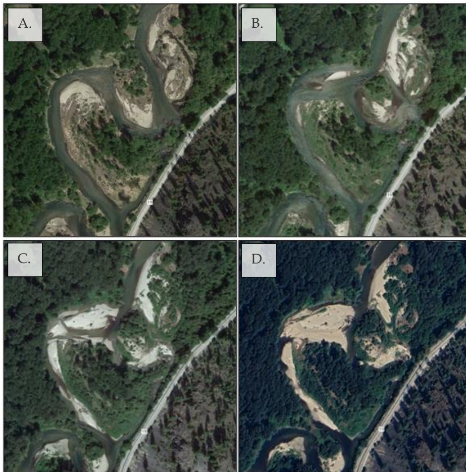
Figure 46. Progression of channel avulsion at RM 20.1 visible in Google Earth aerial imagery: A) pre-avulsion channel alignment with tight meander at RM 20.1 intact, May 2015; B) channel alignment following neck cutoff, July 2017; C) original main channel filling with sediment following neck cutoff, August 2022; D) present-day channel alignment with majority of flow through former side channel on river left, and former main channel mostly plugged with sediment, August 2024.
