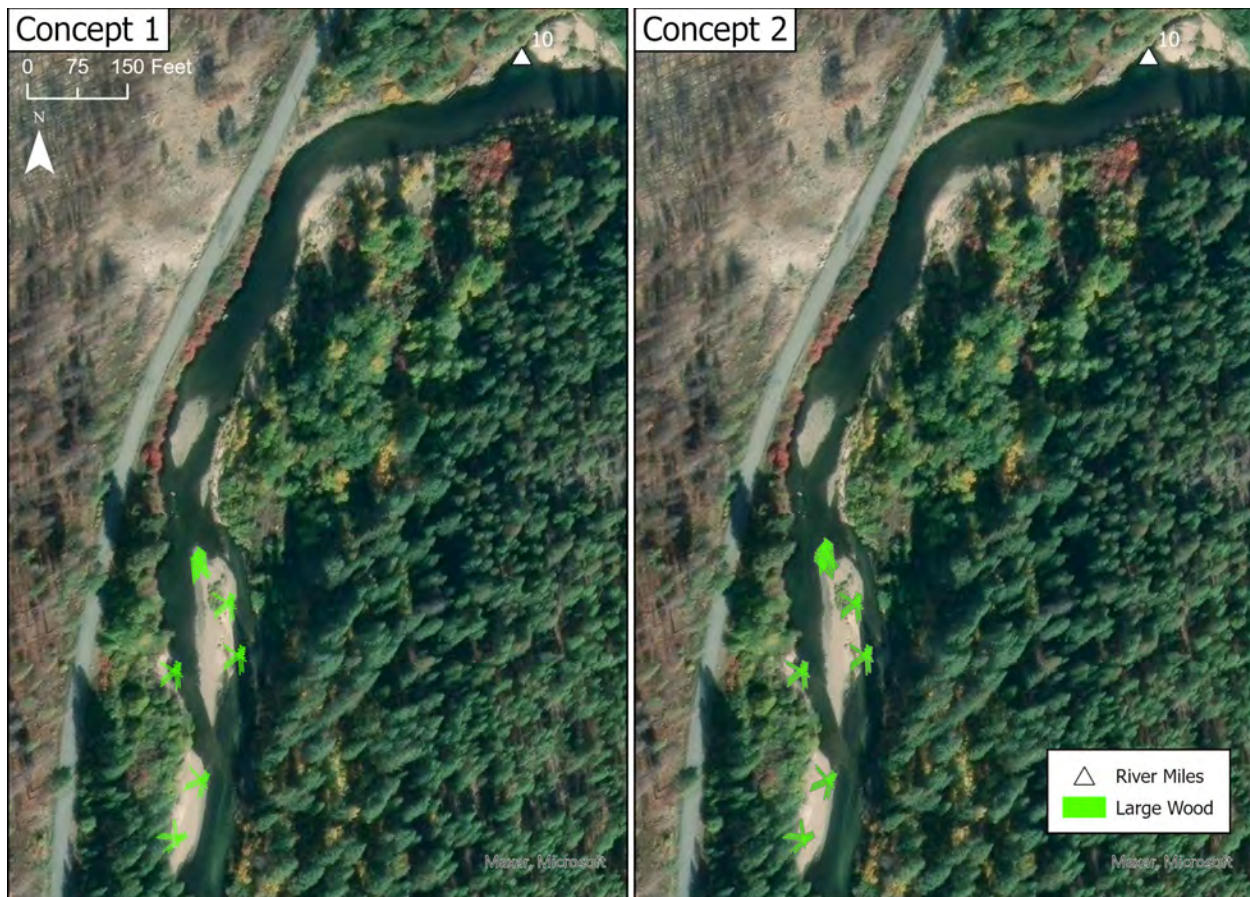
Figure 24.—Example of differences between Concept 1 and Concept 2 designs for RM 10 to 9.5. The only difference between these two concepts is a slightly larger apex structure.
