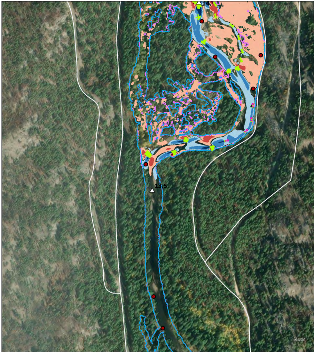
Design 2 vs existing velocity difference with inundation extents (Design 2 minus existing - 10yr flow)
