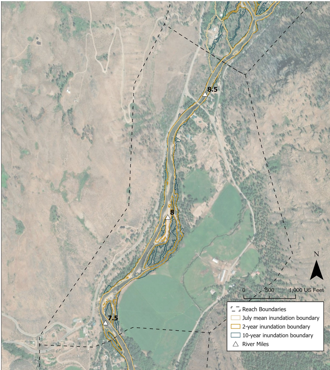
Figure 54.—Inundation boundaries for the July mean, 2-year, and 10-year flows in Perrygin 7.
