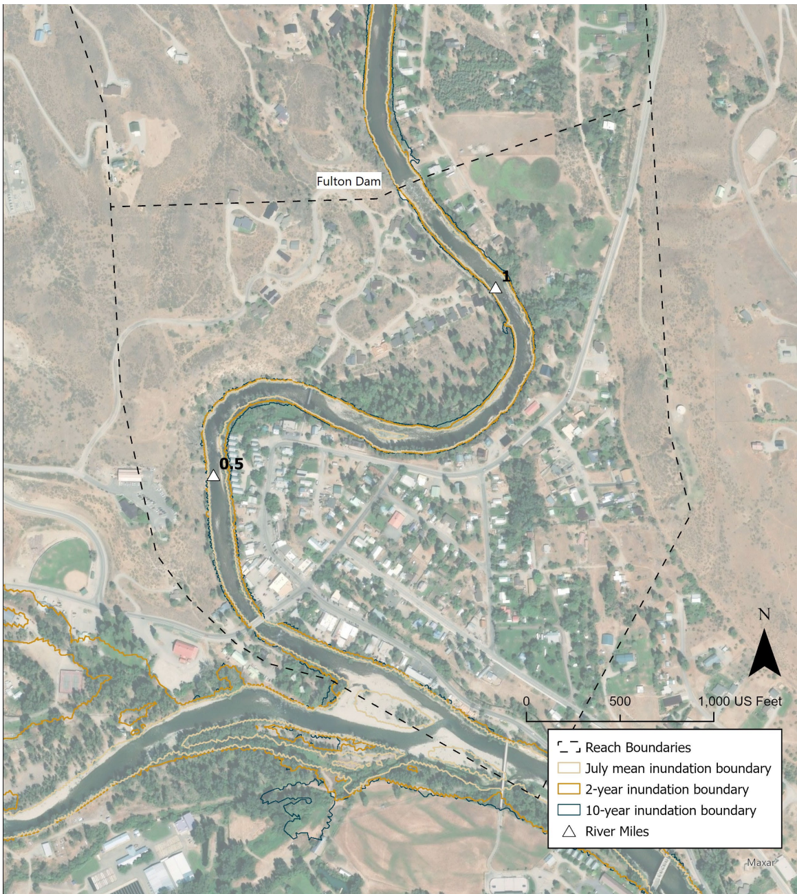
Figure 73.—Inundation boundaries for the July mean, 2-year, and 10-year flows in Perrygin 1.
