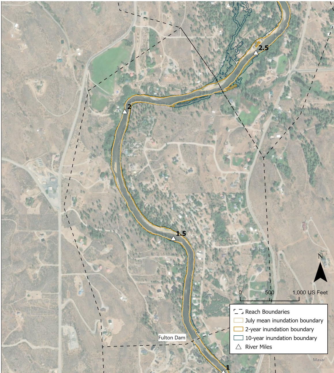
Figure 70.—Inundation boundaries for the July mean, 2-year, and 10-year flows in Pearrygin 2.
