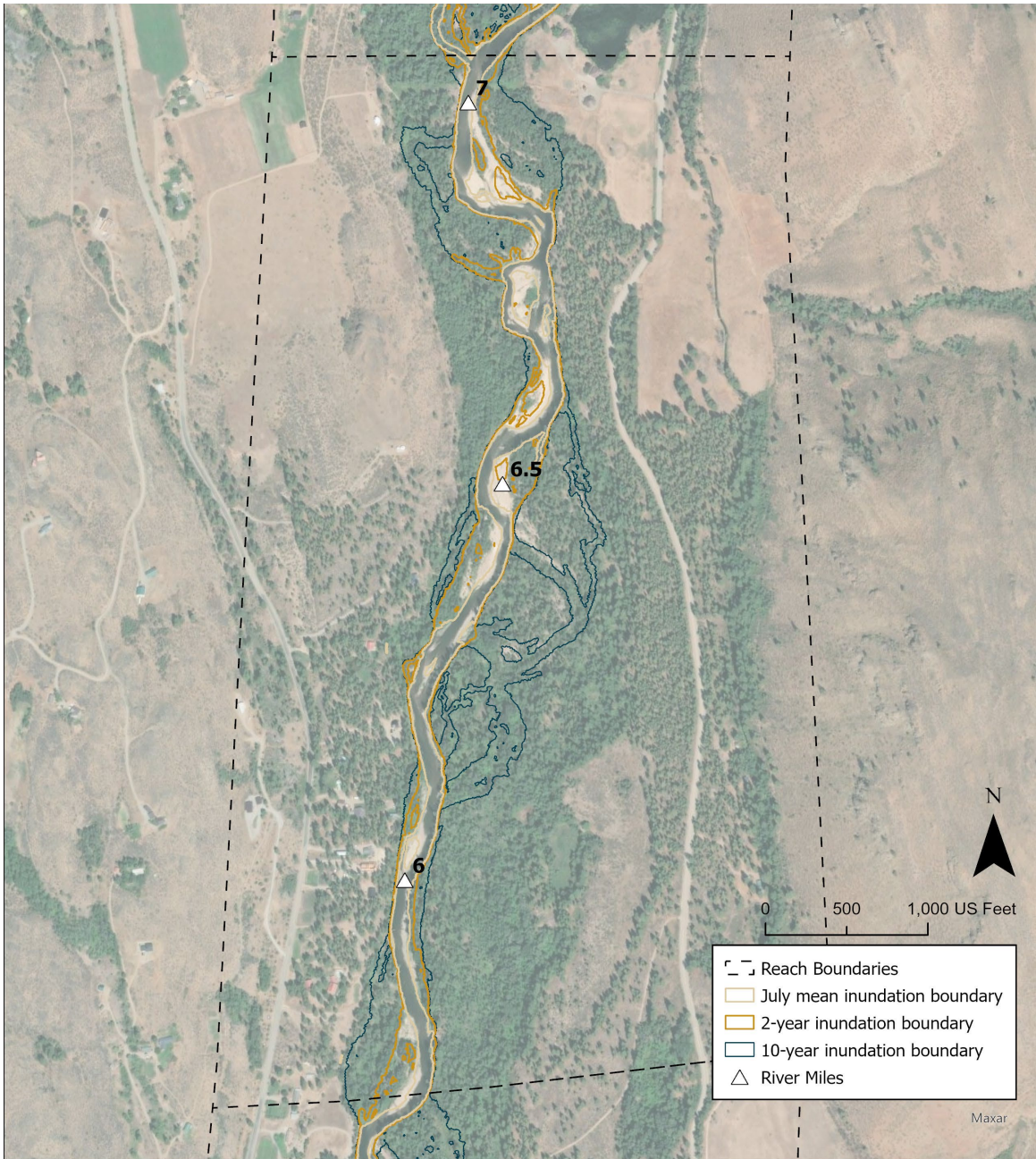
Figure 60.—Inundation boundaries for the July mean, 2-year, and 10-year flows in Pearrygin 5.
