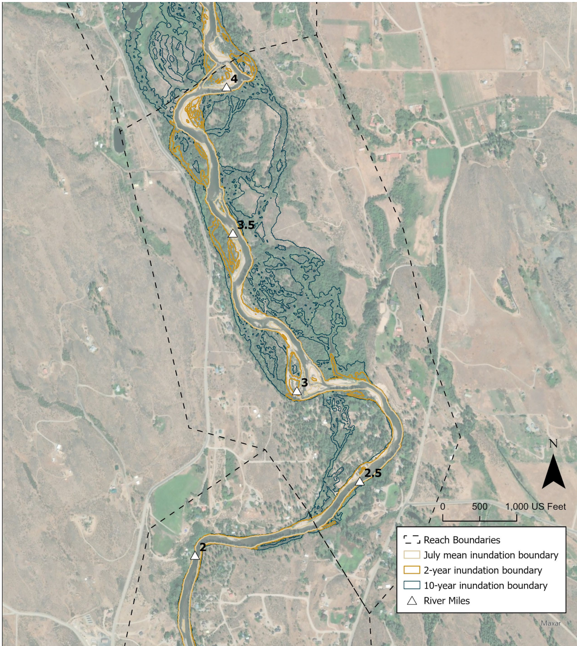
Figure 67.—Inundation boundaries for the July mean, 2-year, and 10-year flows in Perrygin 3.
