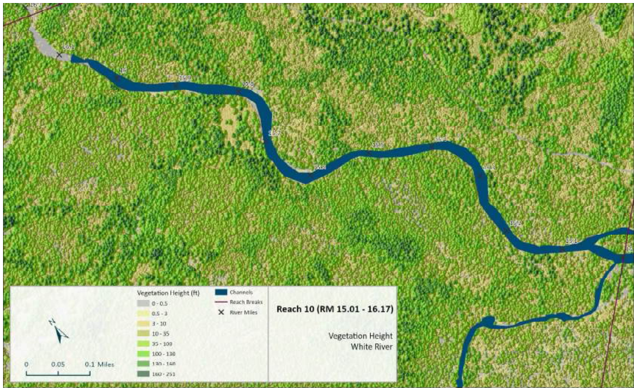
Figure 185. White River, Reach 10: Map of vegetation height classification analysis (LiDAR – based analysis).
