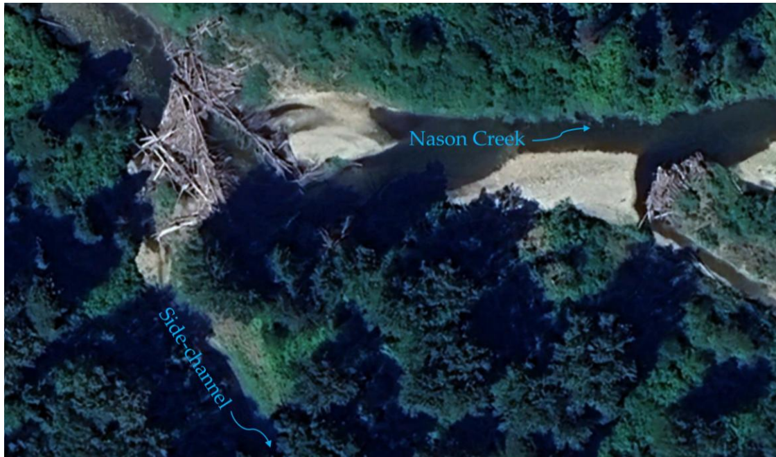
Figure 58. Channel-spanning jam (partly constructed) at RM 2.25 and constructed apex jam downstream. Spanning jam is helping to keep the river-right side-channel active (Google Earth 2024 image).
