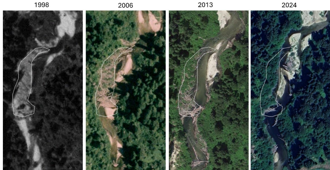
Figure 55. Evolution of channel-spanning log jam near RM 2. Photos series obtained from Google Earth imagery.
