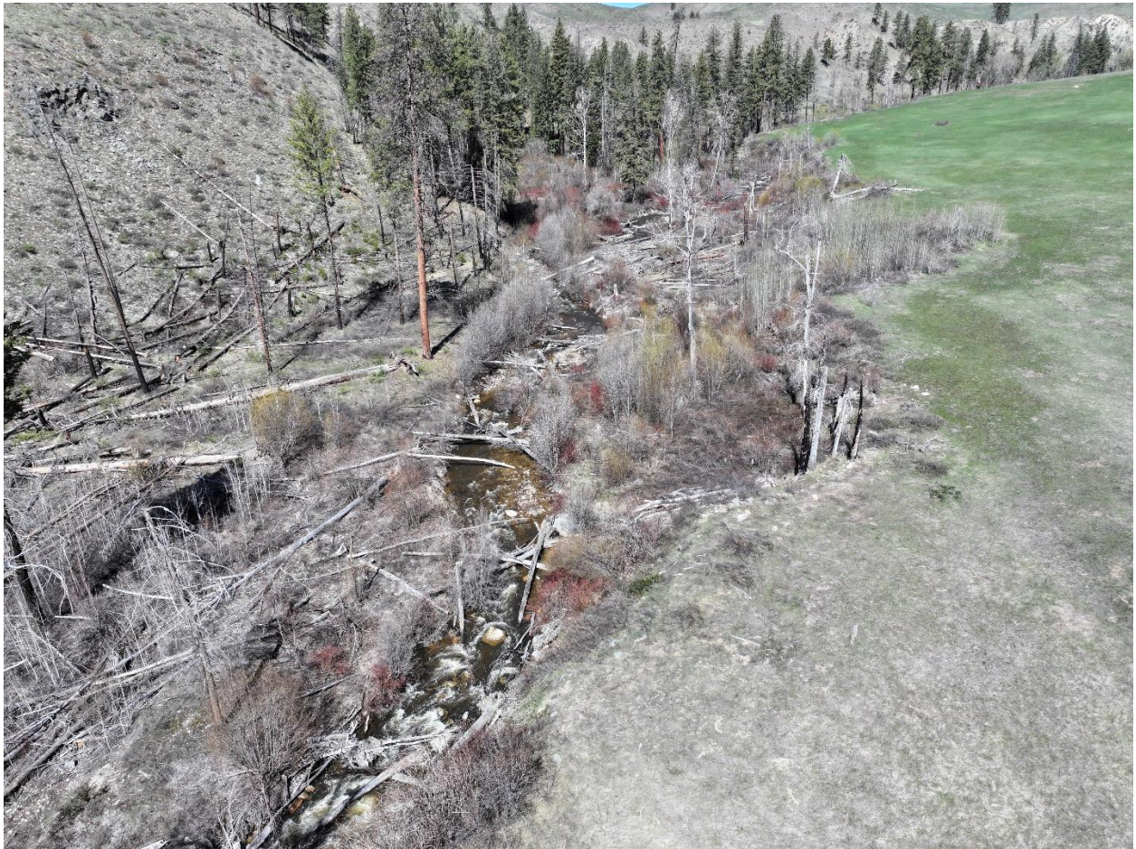
Aerial photograph showing available inset floodplain, channel incision, evidence of past disturbance, and lack of mature riparian vegetation.
