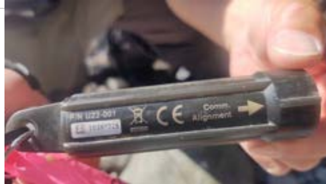
Water temperature data logger that was used for the project. Brand and model: HOBOTemp Pro V2 ONSET U22-001
