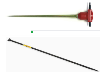
Figure 3a,b. shallow water seismic geophone and seismic source
